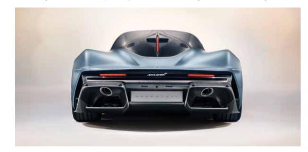
The teardrop-shaped cockpit and aerodynamically optimised body are the foundation for the exceptional aerodynamic drag efficiency, with innovative features such as carbon fibre front-wheel static aero covers, retractable digital rear-view cameras (in lieu of mirrors) and patented active rear ailerons furthering contributing to the ultra-low drag achieved.
