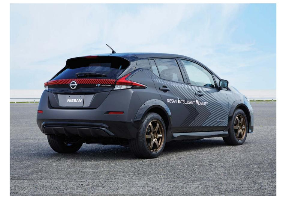
Using separate front and rear electric motors, the powertrain generates 227 kilowatts of maximum output and 680 Nm of maximum torque. This output is complemented by the ultra-high-precision motor control provided by Nissan's advanced EV technology which offers highly responsive, yet uncommonly
