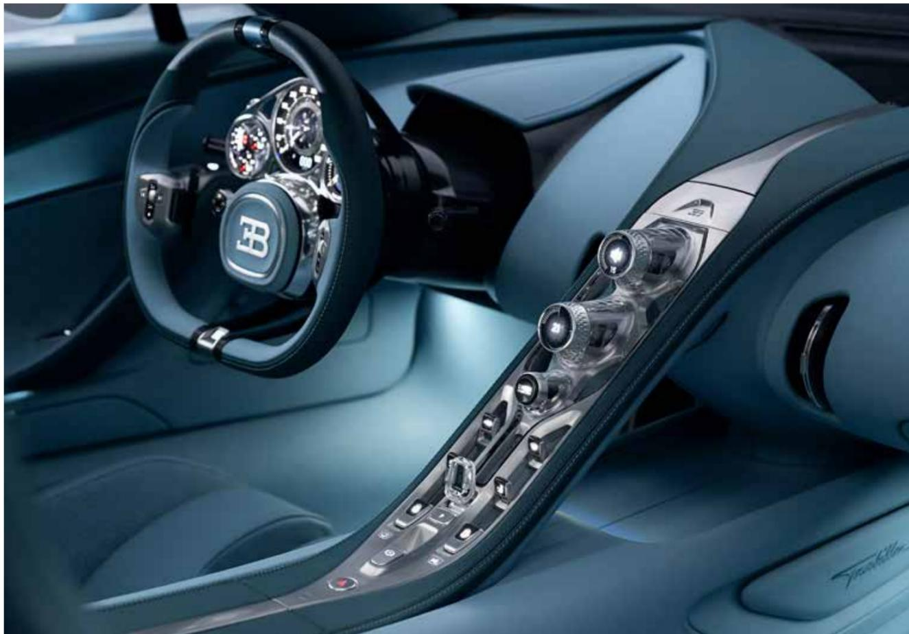
easily date – especially large digital screens – so it's important that it uses as many timeless components as possible. The Tourbillon therefore utilizes a number of design and engineering techniques that will never age, including a completely analogue instrument cluster crafted by Swiss watchmakers and finished with the same care and attention you find in the world's greatest timepieces. Just as these become heirlooms over generations, the Tourbillon is designed as a car for eternity.
